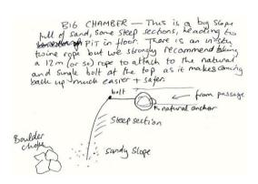
15m rope and 1 hanger+maillon needed for climb down into Big Chamber. Pitch is backed up from wedged boulder in floor of passage. Bolt for hanger was put in 2013 and is in the right-hand wall at around head height.
