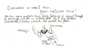
6. 15m rope and 3 hangers+maillons needed for (Not the Stal) Pitch. 1990s bolts (on the right at floor level) found to be in bad nick in 2013. New bolts placed higher up on the right wall and a further bolt put in a few feet down for a re-belay.
